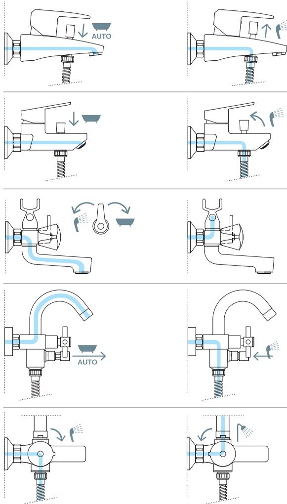
**UGRADNJA BATERIJA****INSTALING THE MIXERS****UGRADNJA ARMATURA****VGRADNJA BATERIJ****ИНСТАЛИРАЊЕ
